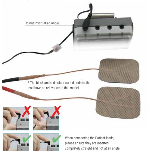
Pushing at an angle may bend the pins.
